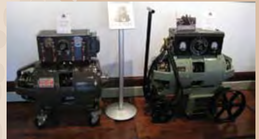
Above: Motor generator welding machines, the left one built in 1928 and the right one built in 1930.
