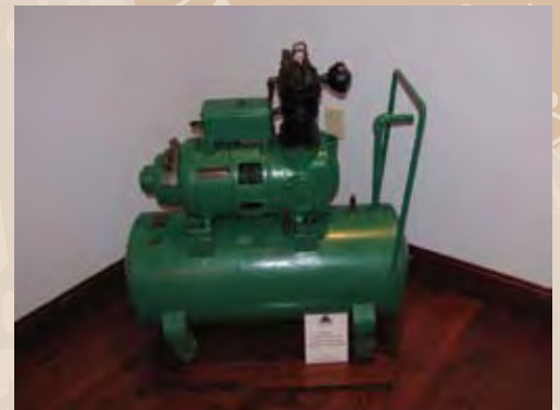
Above: Portable electric compressor for painting and inflating tires, built in 1928.
